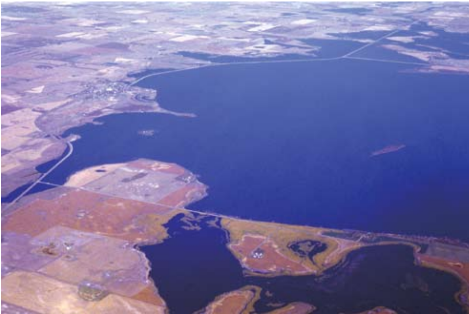
Figure 12. Aerial view of Devils Lake's West Bay. The town of Minnewaukan appears in the upper left-hand corner of the photo. U.S. Highway 281 proceeds north out of Minnewaukan and crosses the west end of the lake before intersecting with State Highway 19 and continuing north. U.S. Highway 281 was kept open by raising the roadbed and riprapping its shoulders. The highway was later relocated farther west, away from the lake. Photo by the author, October 9, 2004.
